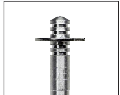
Location of C-clip on jet needle determines mid-range fuel mixture.
